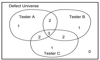
Figure 1: Venn diagram of a defect universe and how 3 different test technologies may cover it. The number of testers that may test a given defect are shown.
