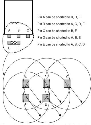
Figure 2: Five pins on two devices and their shorting properties for a given shorting radius.
